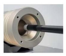
Dual-tip probe arms (optional) for automated top/bottom measurements
