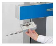
Easiest change of the probing systems thanks to the quick-change adapter
