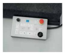
Control panel Movecontrol for comfortable operation of the measuring systems
